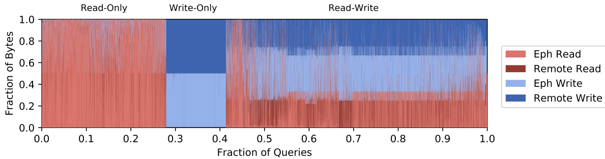
Figure 4: Persistent data I/O traffic distribution between ephemeral storage system and remote persistent data store. Each vertical bar corresponds to a query, the four colors correspond to read/write from ephemeral/remote systems, and the y-axis represents the fraction of total persistent data that was served by the corresponding storage system. Queries are sorted, within each class, in decreasing order of number of persistent data bytes read/written. Discussion in §4.2.
